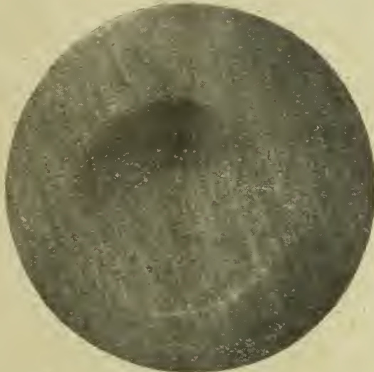
Fig. 5.—Brinell impression \times 20 .
